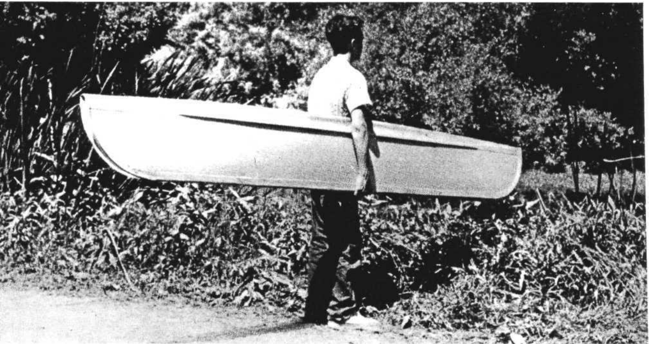
This kayak weighs only 40 lbs. and folds down the middle so that you can carry it easily. Note the bottom rub rail which protects the canvas. You can carry a fleet on your car
